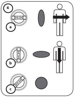
Fig. 6a vertical flat spray pattern: For spray movements from left to right
