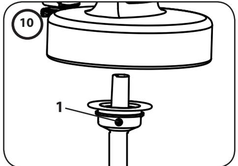
**CAUTION!** Never clean seals, nozzles or air holes of the spray gun with metal objects..
